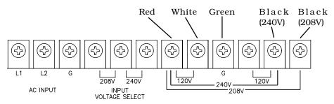
(Note: This diagram shows the terminal block of a SU6kVA model. SU10kVA models have double connectors, but the wires are attached to the same terminals on both models.)
